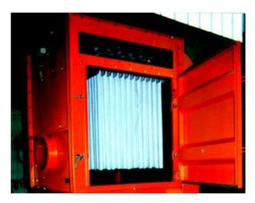
ULTRATUB Compact Filter are made from filter tubes which can be placed individually or lined up in special rails.
