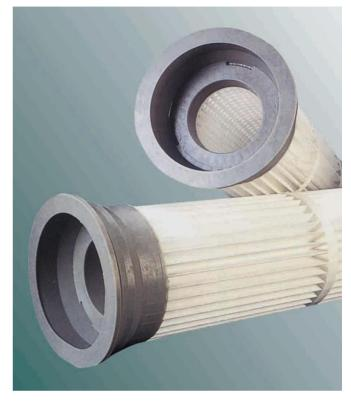
**ULTRASEP** filter cartridges made from a 100% spun bond polyester fabric have a very open and pleat structure with a small pleat depth. This design prevent particles from penetrating into the structure and realizes a significant increase of the dust collection capacity (BIA class M, e.g. emission grad < 0.1%) with a constant low differential pressure level.
